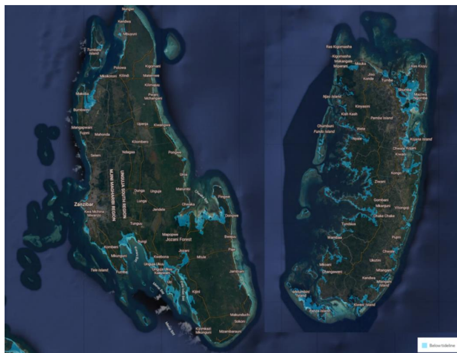
Figure 7. Inundation map for both of Zanzibar islands under the emission scenario SSP5-8.5 of a sea level rise of 80 cm until 2100
